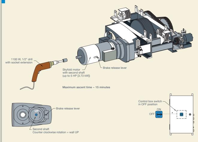
In the unlikely event that the Skyfold wall does not respond to the key switch operation, it can now be operated by using a heavy duty drill. A shaft extension has been added to the motor allowing for an alternative method of raising and lowering the wall. This feature is now standard on all of our walls. This diagram is for illustration purposes only. Please refer to the applicable operating procedures for complete instructions.
