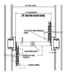
Eliminate the need to remodel your hallways in order to meet California OSHPD requirements. Our flush exit device on 7' - 9" pairs or double egress pairs creates a 44" opening clearance per door.
